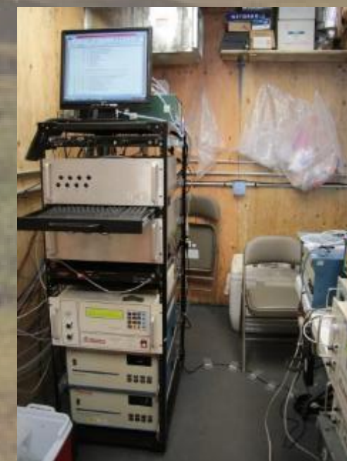
GEM: Tekran 2537 Air Hg Analyzers, \text{CO}_2 , \text{CH}_4 , \text{O}_3 , \text{NO}_x , \text{O}_2 )
